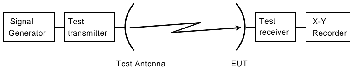
Figure 10: Test arrangement - antenna transmit radiation pattern measurement
