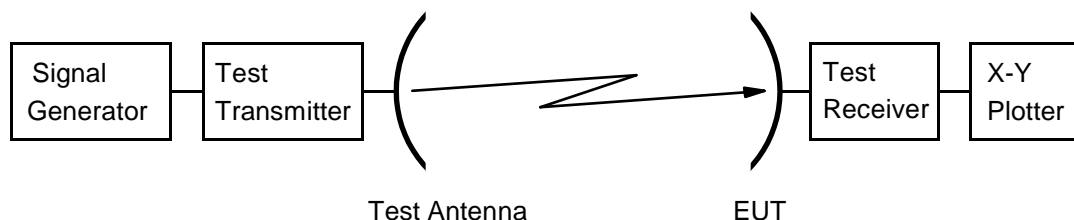
Figure 9: Test arrangement - antenna transmit radiation pattern measurement
